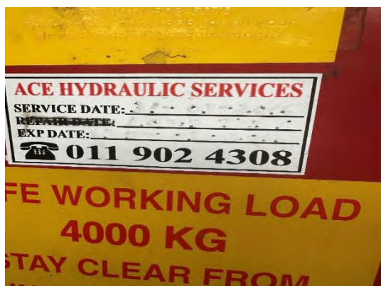
Figure 2: Un-serviced car lift
